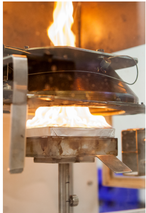
Cone calorimeter testing
