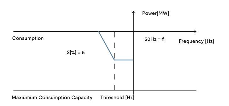
Active power frequency response in under-frequency with 5% drop
