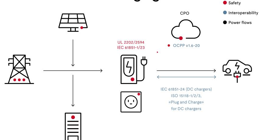
G2V: Grid-to-Vehicle CPO: Charge Point Operator OCPP: Open Charge Point Protocol
