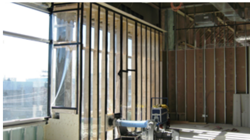
Figure 11: Interior test chamber used to test a portion of curtain wall section
