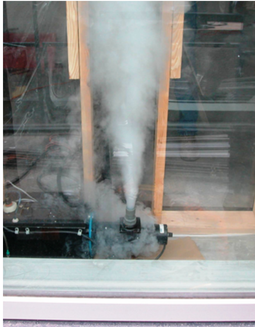
Figure 16: Portable smoke generator used to fill test chamber with white smoke
