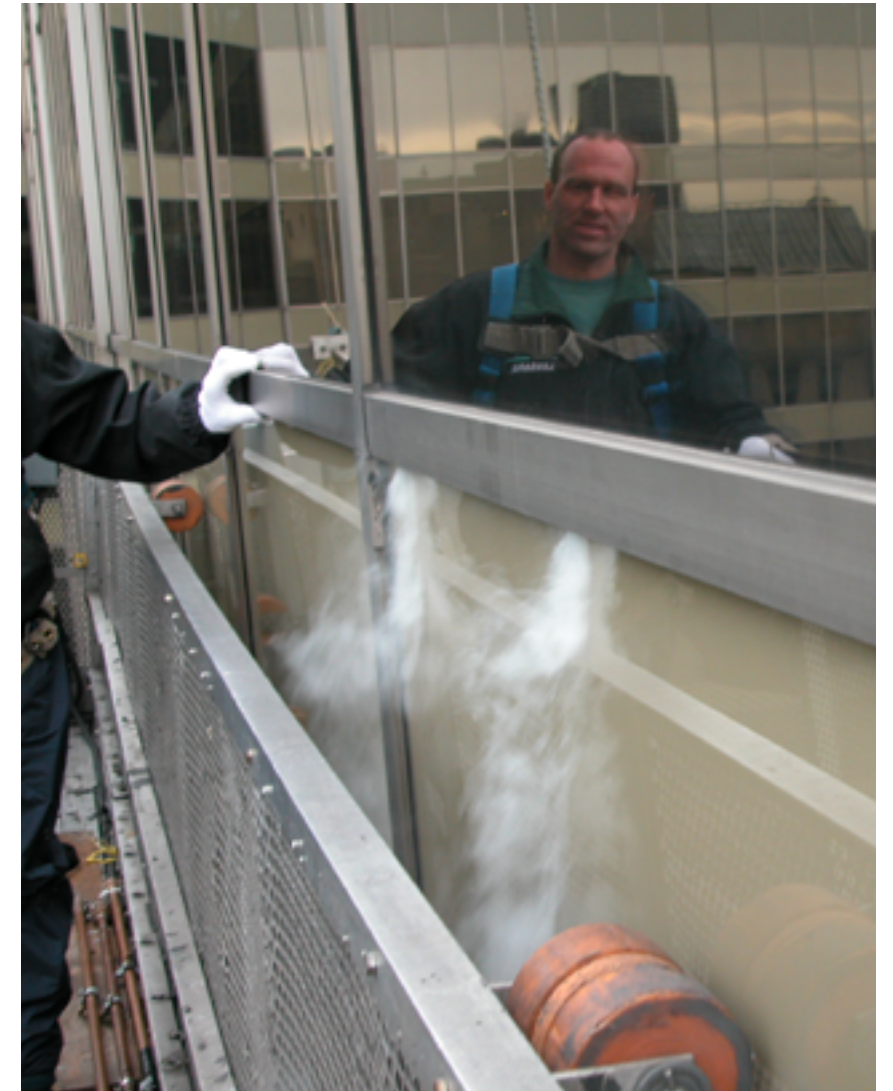
Figure 17: Excessive smoke exfiltration visible on exterior side of curtain wall test specimen
