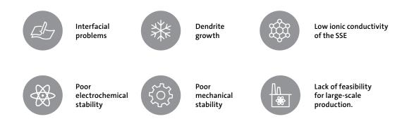
These problems can cause poor performance and limit their application scope. Among all the key problems mentioned in the list above, interfacial problems and dendrite growth can cause significant impacts on performance and safety.
